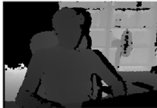
**Fig. 2.** Grayscale depth image. Each pixel demonstrates its distance from camera
