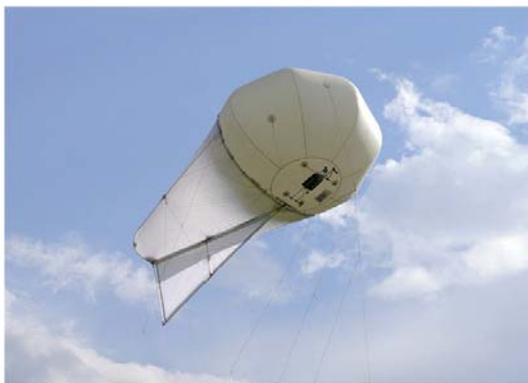
**Fig. 3.** Colibris hybrid aerostat developed at OSKBES MAI [11]
