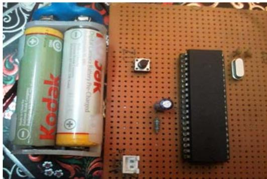
Fig. 3. Voice IC Board connection
