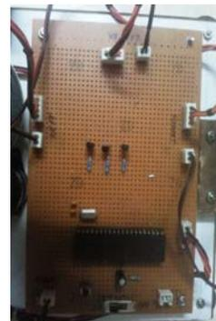
Fig. 2. Supply connection to the microcontroller
