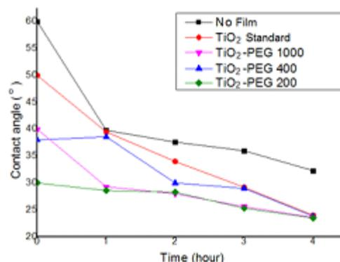
**Fig. 2.** Contact Angle Measurement
