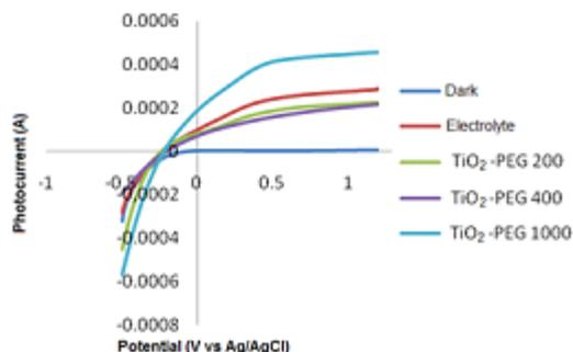
**Fig. 3.** LSV of  $\text{TiO}_2$  + PEG electrode with illumination, an electrolyte solution of 0.1 M  $\text{NaNO}_3$
