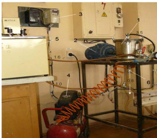
**Fig. 1.** Scheme of experimental laboratory installation
