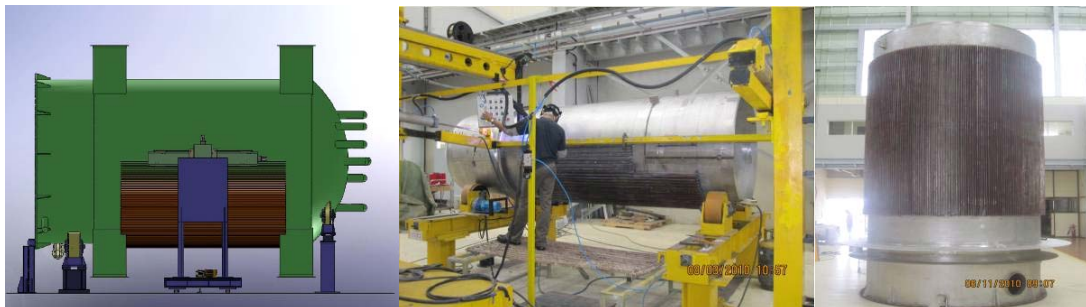
Fig. 5. Braze welded fins in SSFC cold traps along with automation set up
