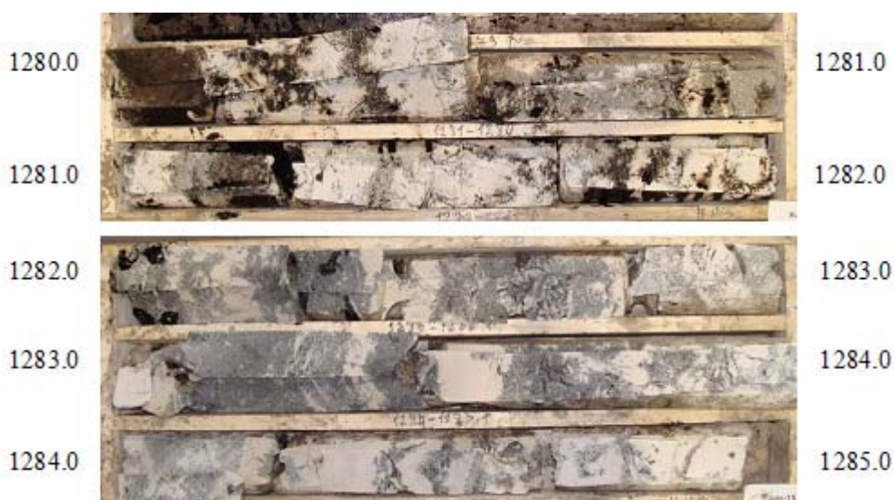
Fig. 2. Core sample from the zone of the water-oil contact
