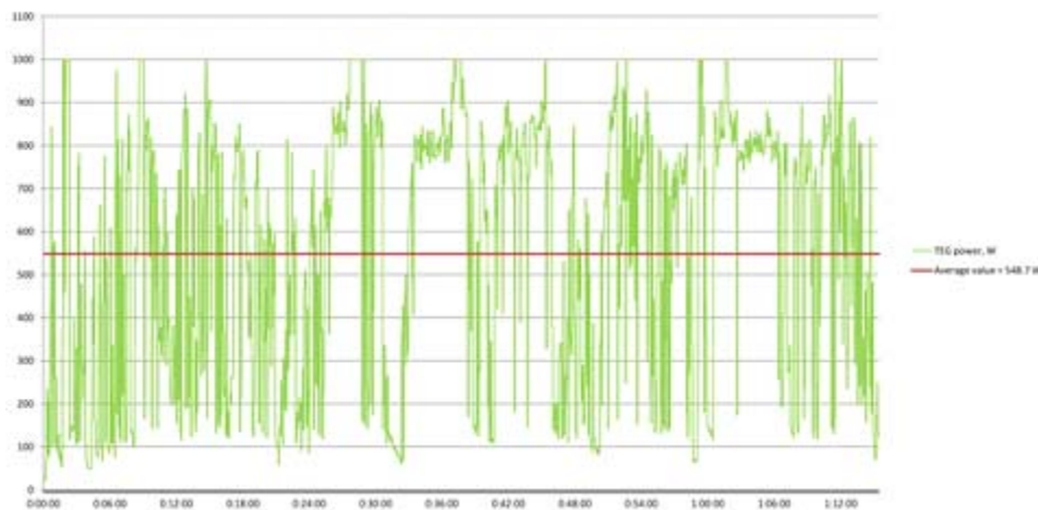
Fig. 7. Graph of the calculated TEG output during the drive along the route #1 Nizhny Novgorod - Lyskovo
