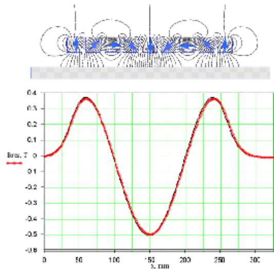
**Fig. 4.** Flux-lines pattern and on-core-surface normal flux-density distributions of the field produced by Halbach PM-system
