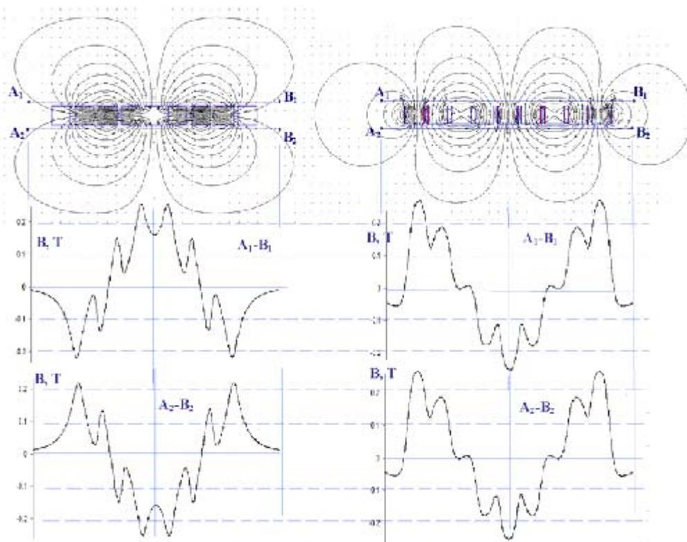
**Fig. 5.** Magnetic fields and flux-density normal component distributions along the straight contours above and underneath Halbach array. Magnetic field patterns and plots are obtained using the *FEM*-models of *x*- and *y*-current layers of PM Ampere-models.
