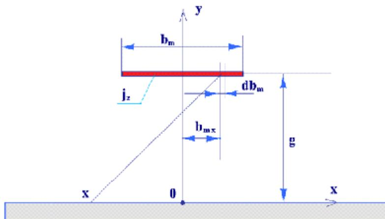
**Fig. 2.** Current layer with linear current density  $j_z$  located above the core
