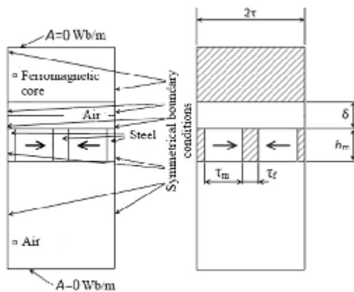
**Fig. 6.** The finite-element model, materials and boundary conditions
