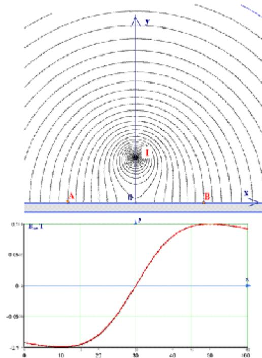
**Fig. 1.** Magnetic field pattern for the case of thin current-carrying conductor located above the flat ferromagnetic core and plots of the normal flux-density component determined on the *AB* part of the core. Both analytical (calculated by (4)) and *FEM*-modeling results are presented (both plots practically coincide).
