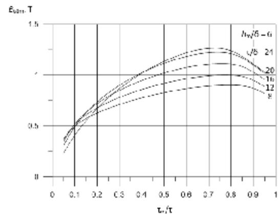
**Fig. 7.** Plots of the amplitude of the first harmonic of the magnetic flux density at  $\alpha = 1 \text{ mm}$  and  $h_m/\phi = 6$  as a function of  $\tau_m/\tau$
