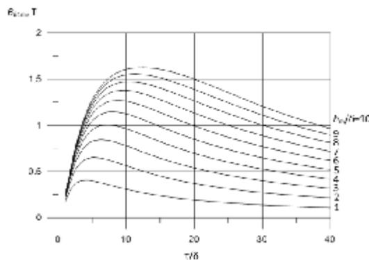
**Fig. 8.** First harmonic amplitude of the flux density vs  $\tau/\alpha$  for different  $h_m/\alpha$  (at  $\alpha = 1$ )
