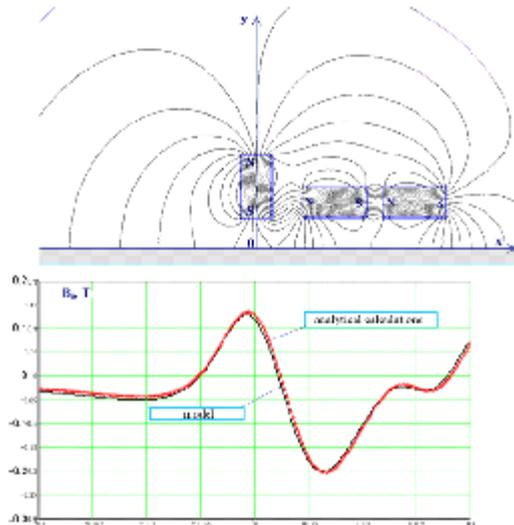
**Fig. 3.** The normal component of flux-density distribution of the field produced by the PM-system on the surface of flat core
