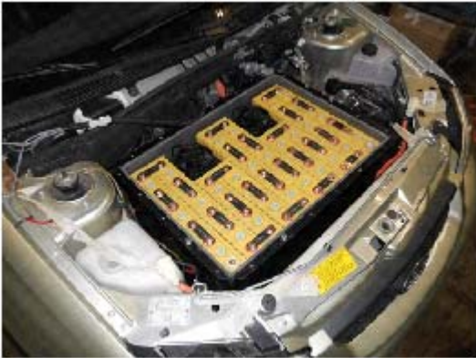
Fig. 8. Electric energy storage system in the underhood space of the vehicle's experimental prototype
