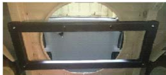
Fig. 6. Mounting of the subframe to the load-bearing elements of the body
