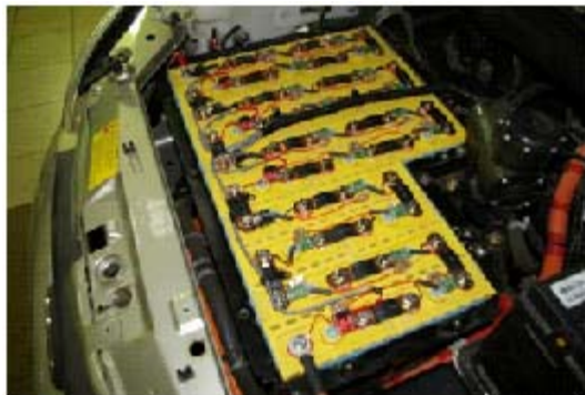
Fig.2. a) the first block of accumulator cells; b) position of the second and the third blocks of accumulator cells
