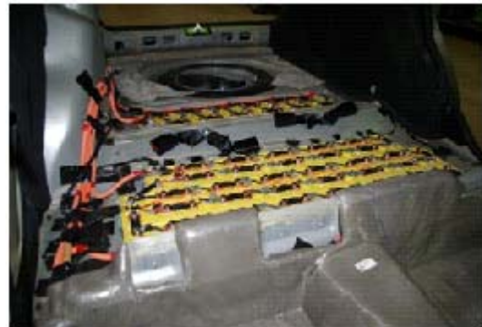
Fig.2. a) the first block of accumulator cells; b) position of the second and the third blocks of accumulator cells
