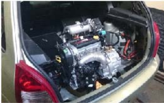
Fig. 5. Position of the Range Extender in the vehicle
