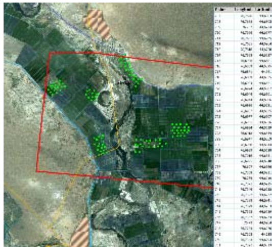
Fig. 3. Measurement points of soil electrical conductivity values and NDVI of crops on the test sites and the database fragment with points' coordinates
