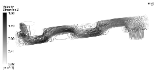
Fig. 3. Lines of flow in a heat exchanger with segmental baffles.
