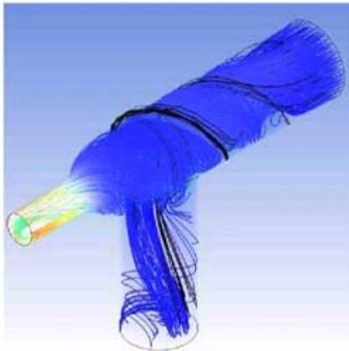
Fig. 5. Model of assessing the effect of a gas flow with high rarefaction on a swirling dust and gas flow
