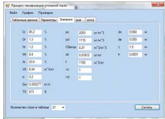
Fig. 2. Data-entry window for entering the initial programme data for gasification in the flow
