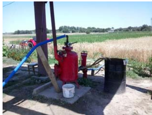
Fig. 2. Water cleaning and additional fertilizing system
