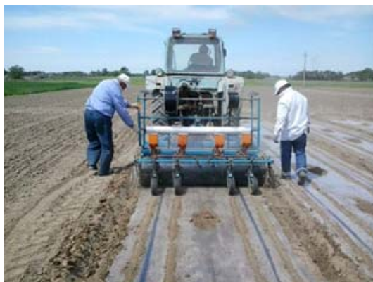
Fig. 3. Double-row rice sowing with laying of both irrigation tape and tensioning of the film
