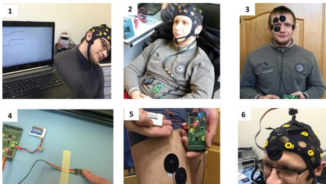
Fig. 1. Methodology of testing: 1) motor activity; 2) EEG; 3) EOG; 4) PPG and SpO 2 ; 5) EMG, 6) thermometry
