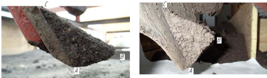
a) Soil wedge on the working surface of the rotary tillage tool with shovel shaped tines for incorporating the weed seeds;
