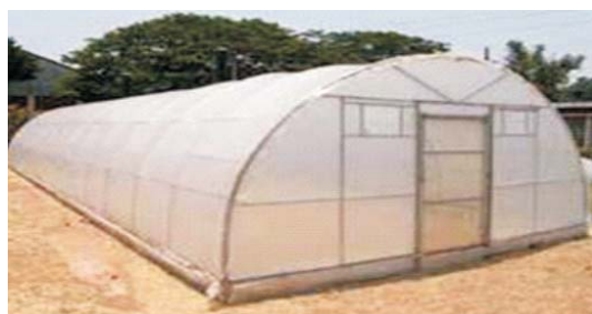
Fig. 1. Solar Tunnel Drier
