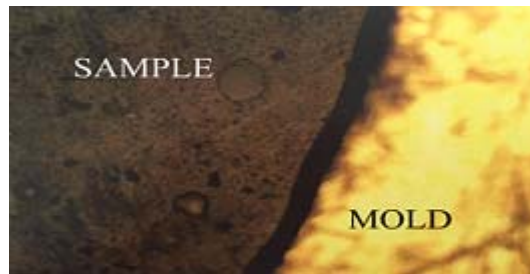
Fig. 2. Gap formed between mould and the sample (linear shrinkage) at 80 x magnification
