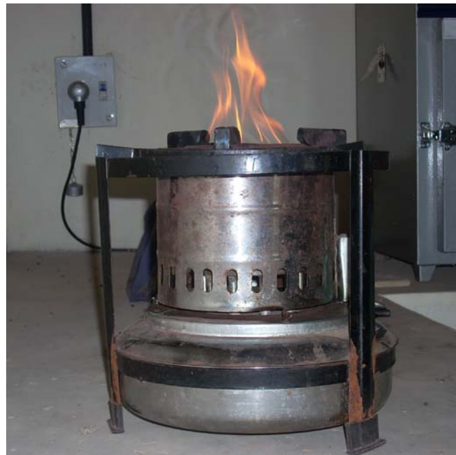
Fig. 4: Biodiesel operated wick stove
