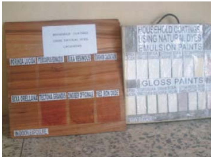
Fig. 2: Application of the surface coatings on wooden and concrete slabs
