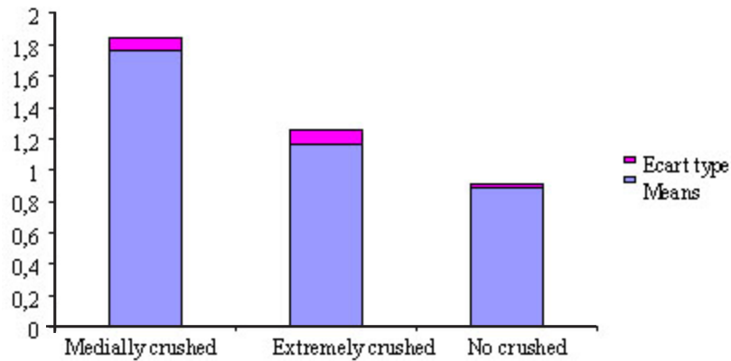
Fig. 2: Variability of extraction yield of Eucalyptus leucoxyton in accordance with crushing
