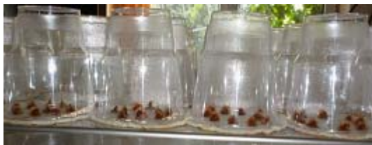
Fig. 3. The important stage is the viability test (germination of seeds before their preservation) The device for the seed germination test ‘APS-2M’ (Jacobson’s table)
