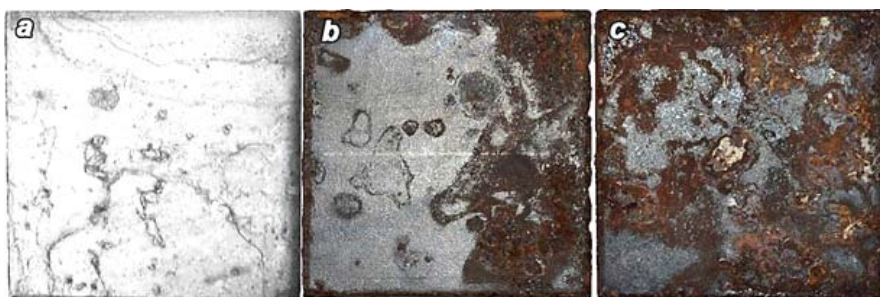
Fig. 3. Corrosion damage of test metal coupons placed in "red type" of HGIO: a – before the experiment; b – after 2 months; c – after 4 months
