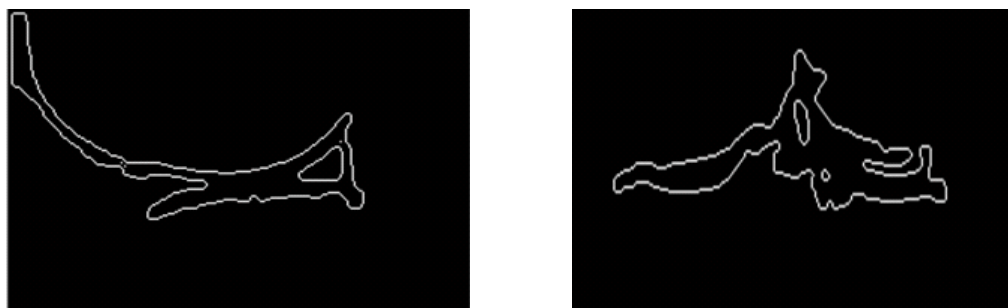
Fig.13. Canny edge detection of the binary image obtained previously (a) sagittal plane (b) coronal plane
