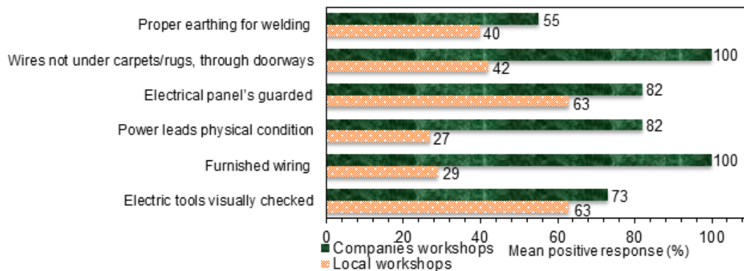
Fig. 4. Comparison of mean positive response rates of electric safety in surveyed LWs and CWs. The variables shown in y-axis are referred to OSH items of the studied element. The higher the mean positive response the best is the compliance referring to any particular OSH element. The OSH elements showing overall mean positive response (above 50%) were all in acceptable range. However, the values (below 50%) were considered as serious and required further actions for improvements of the concerning OSH element
