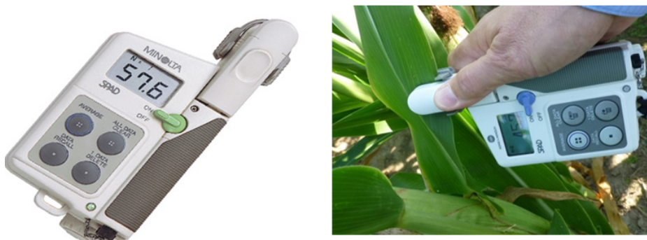
Fig. 1. Measure the chlorophyll content of the leaves using a chlorophyll meter
