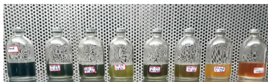
Fig. 1. Various colour changes observed in the bromocresol green media
