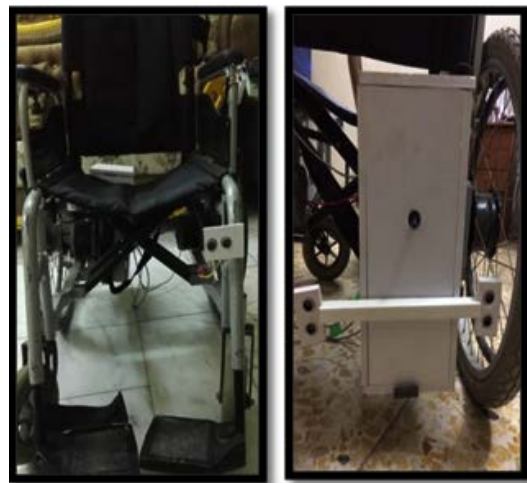
Fig. 8. The ultrasonic sensor location (a): front view (b): back view
