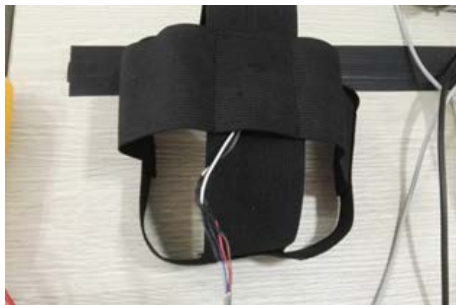
Fig. 7. Gyroscope sensor placement
