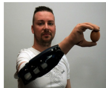
Fig. 10. Myoelectric prosthesis involve high technology and enables composite and complex hand movements
