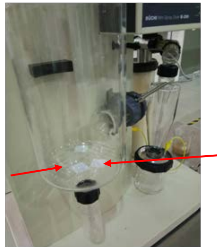
Fig. 2. The Borosilicate and Teflon plates were placed horizontally in the bottom of drying chamber. The adhesion flux deposited at plates were observed and weighed ( n=3 )
