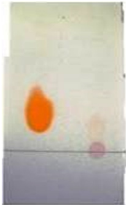
Fig. 2. TLC experiments showing the different R_f values of control dye solution and decolorized samples.
