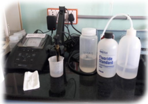
Fig. 1. Thermo Scientific ORION STAR A214 ISE meter used for Fluoride estimation of ground water samples
