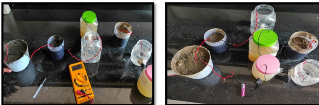
Fig. 8. A [Series setup of all system]; B[whole system connected in series with LED]
