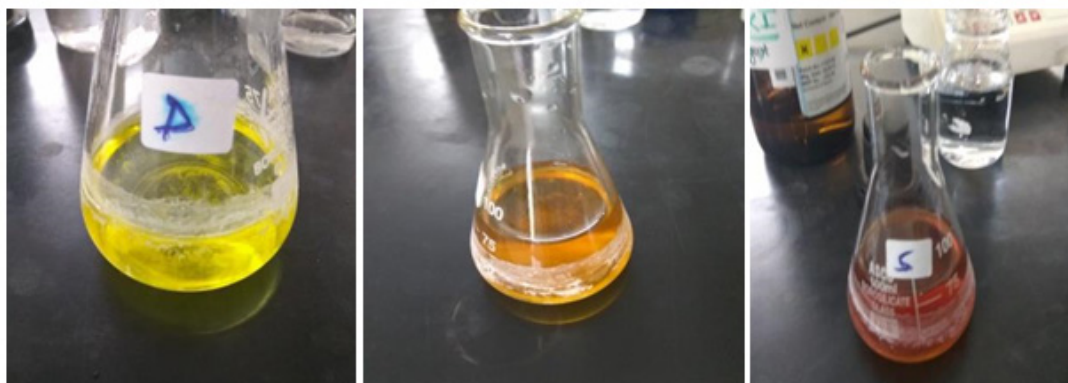
Fig. 1. Colour change observed during synthesis of Ag nanoparticles
