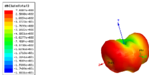
Fig. 20. A three - dimensional pattern of a segment of coaxial cable with four radiating elements
