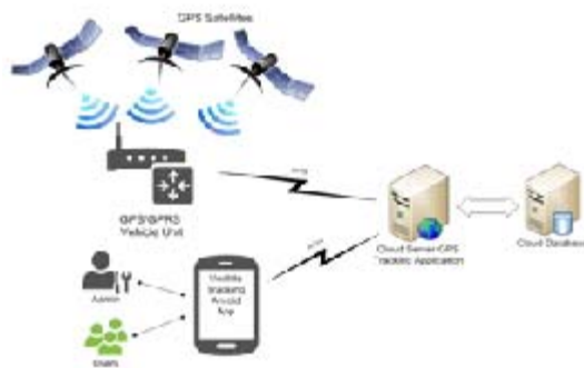
Fig. 2. Architectural overview of proposed system
