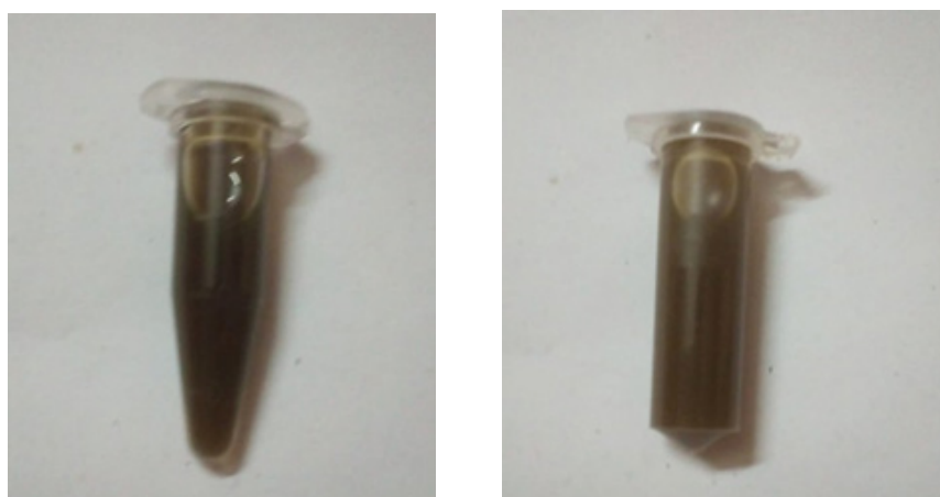
Fig. 5a. Leaf extract of Bryohyllum pinnatum (lam.) with CuCl 2 as precursor 5b. Leaf extract of Polyalthia longifolia (Sonn.) with CuSO 4 as precursor at 24 hours
