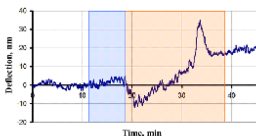
Fig. 3. The relation of relative deflection of sensor cantilever on time during CRP adsorption from the solution with concentration of 50 \mu\text{g/ml}
