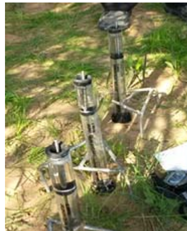
Fig. 2. Mini disk infiltrometer used in the field for measuring unsaturated hydraulic conductivity
