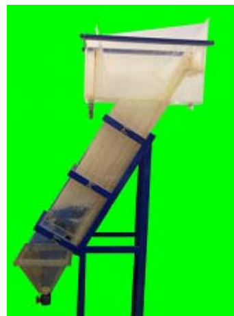
Fig. 5. Inclined settling tank from polymethyl methacrylate (PMMA) with honeycomb blocks having the height of 50 mm and the angle of inclination 60^\circ
