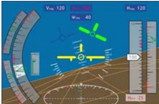
Fig. 2. Avoiding ground strike indication
