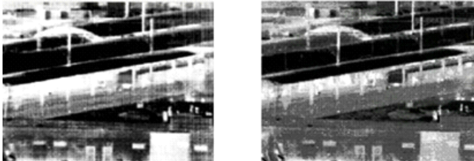
Fig. 6. Example of results of synthesis two-band IR images (an electric train platform) with the two-dimensional histogram equalization (on the right) and with usual association (at the left)
