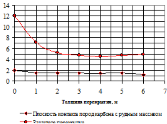
Fig. 5. Dependency of maximal vertical shifts on the thickness of protective cover
