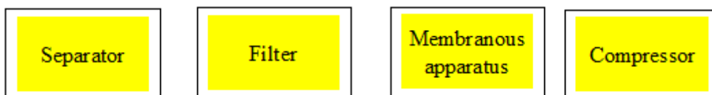
Fig. 6. A principal scheme of the biogas membranous cleaning
