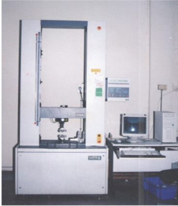
A Lloyd's Universal Testing Machine (United Kingdom) model no. LR 100 K, equipped with a 10 kg tensile load cell
